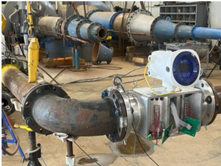
Straight Pipe and Downstream of Ell-0D 90 orientation
